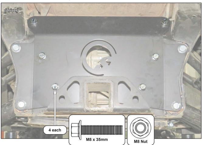
If SuperATV Rear Steer is installed, use this hardware to secure Rear Steer Cylinder Mount to Back Plate (B) and Frame.
