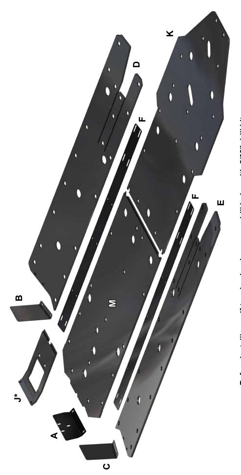
Before installing self-tapping hardware, pre-drill holes with 5/32" drill bit.
