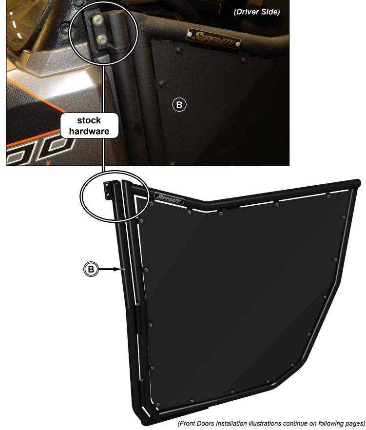
Secure Front Driver Door (B) to Floor with M6-1.0 x 30mm Lg. Bolts. -
