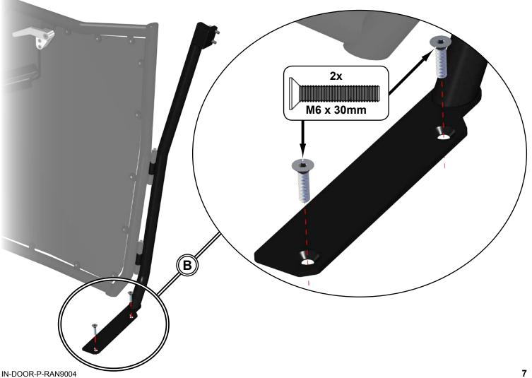
Install Front Striker Bracket (Driver) (F) with hardware shown.
