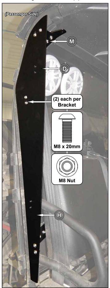
Install Passenger Male Hinge (F) to Passenger Frame Bracket (D) with hardware shown.
