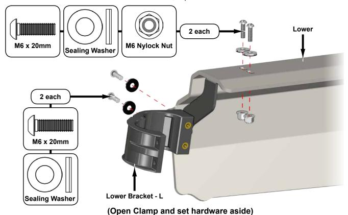
install provided Seal to bottom of Lower as shown
