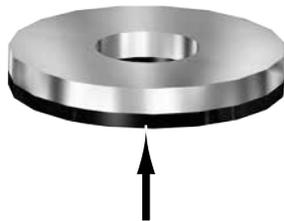
Rubber must face plastic when installing Sealing Washer
