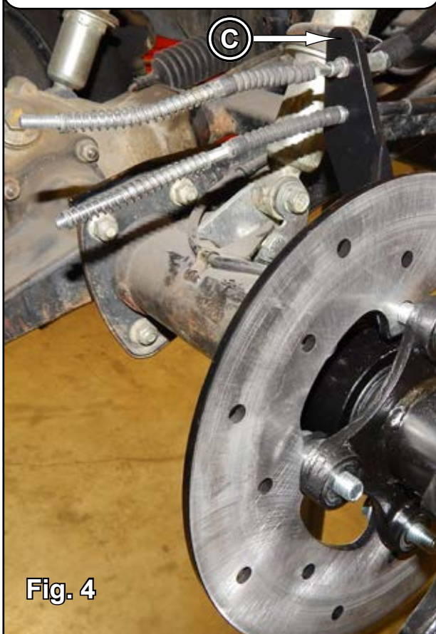
Cables through Brake Line Bracket (C)
