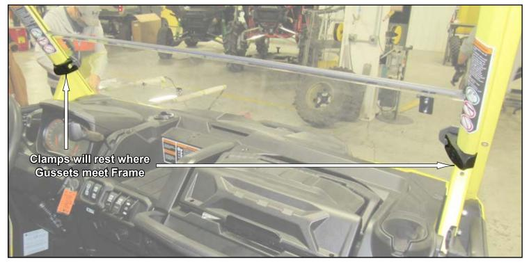
Before drilling holes, check behind area to be drilled for any interference.
