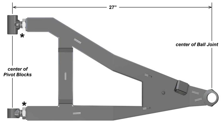
\*Leave Jam Nuts loose. Tighten after final adjustments have been made.
