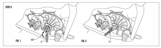
Lift up the handle (7) 90° to depress the belt pulley - you can easily remove and replace the belt.
