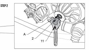
2. Rotate the tool (11) to thread into secondary shaft (2) to figure (A).
