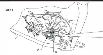
1. Align the positioning flange (8) over the secondary shaft (A) and press down by hand.
