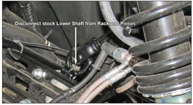
Remove stock, Shafts, Motor, and ECU from machine.
