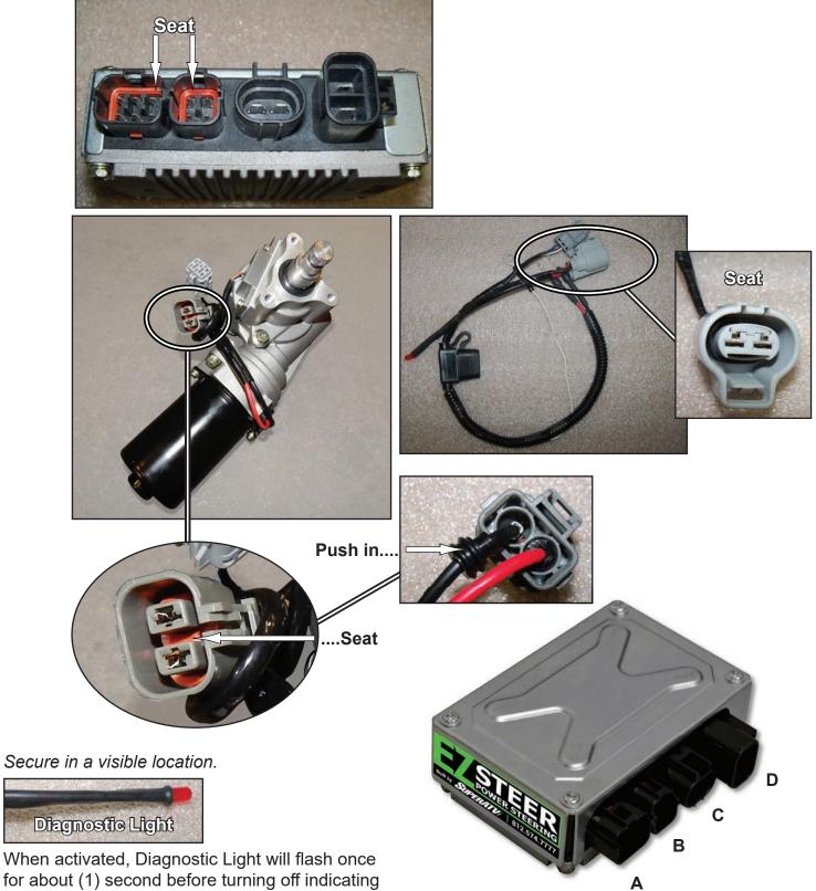
for about (1) second before turning off indicating proper function. Should different patterns occur, contact SuperATV.
