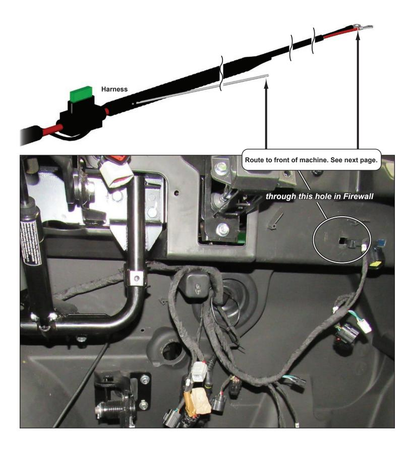
Connect Harness power wiring as shown
